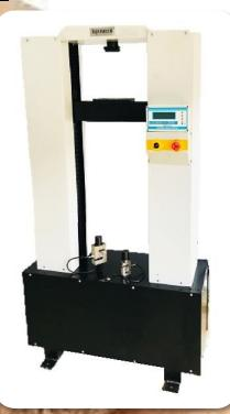
As per various testing standard designed to measure the flexural stiffness and strength properties of polymer matrix composites.
